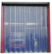
Available in 2mm, 3mm, 5mm thickness and in 200mm & 300mm width for normal and freezer grade Application. Can be supplied with or without Hardware. Also available in Roll form.
